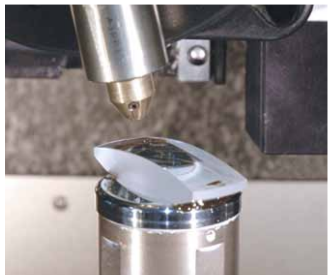
Measuring an aspheric lens segment
