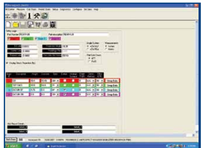
Set Up Program- individual gauges can be associated with measurement features by a simple set up menu
